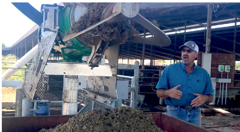
Manure solid separator funded by AMMP at Beretta Dairy in Sonoma County.
