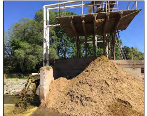
*Screw auger separation of liquid and solids*
